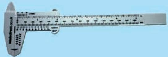
150MM PLASTIC VERNIER IDEAL FOR TAKING MEASUREMENTS OF SEALS AND OTHER COMPONENTS
